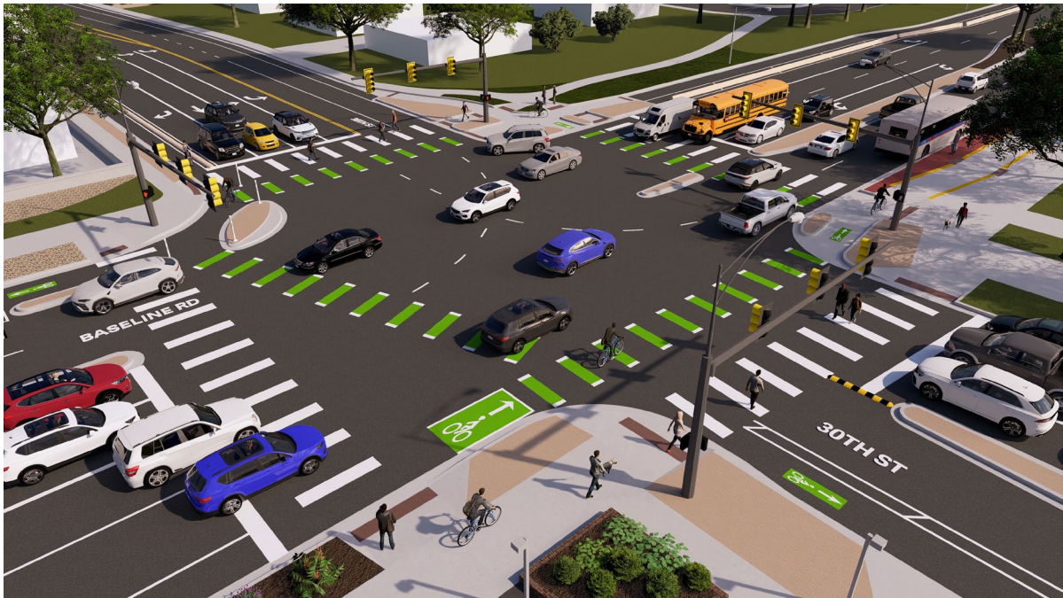
Figure 3: Baseline Road Phase 2 Protected Intersection Design at 30th Street
