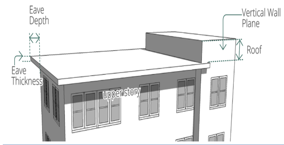
7 8 9 10 11 12 Figure 14-49. Example of a Flat Cap Type
