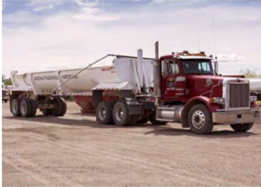
Figure 7 Use more axles to decrease load on delicate road surfaces.
