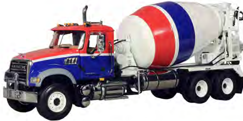
Figure 4 10 cu yard concrete truck
