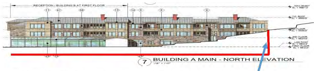
Figure 5 A building underground parking requires a 30 foot retaining wall with revetments to restrain mass movement
