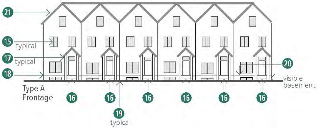
Figure 14-36. Row Building: Facade Design Requirements
