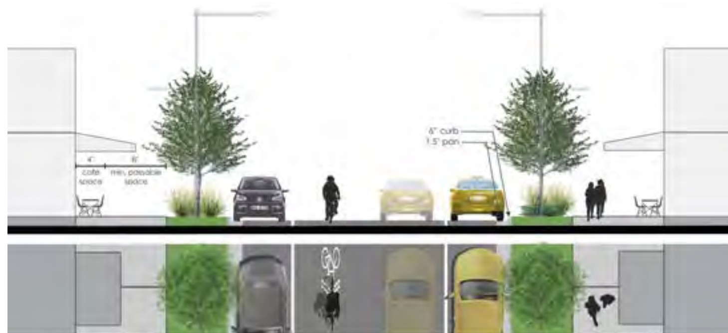
The Activation Street type includes two lanes of traffic, on-street parking, a landscaped buffer with trees and wide sidewalks
