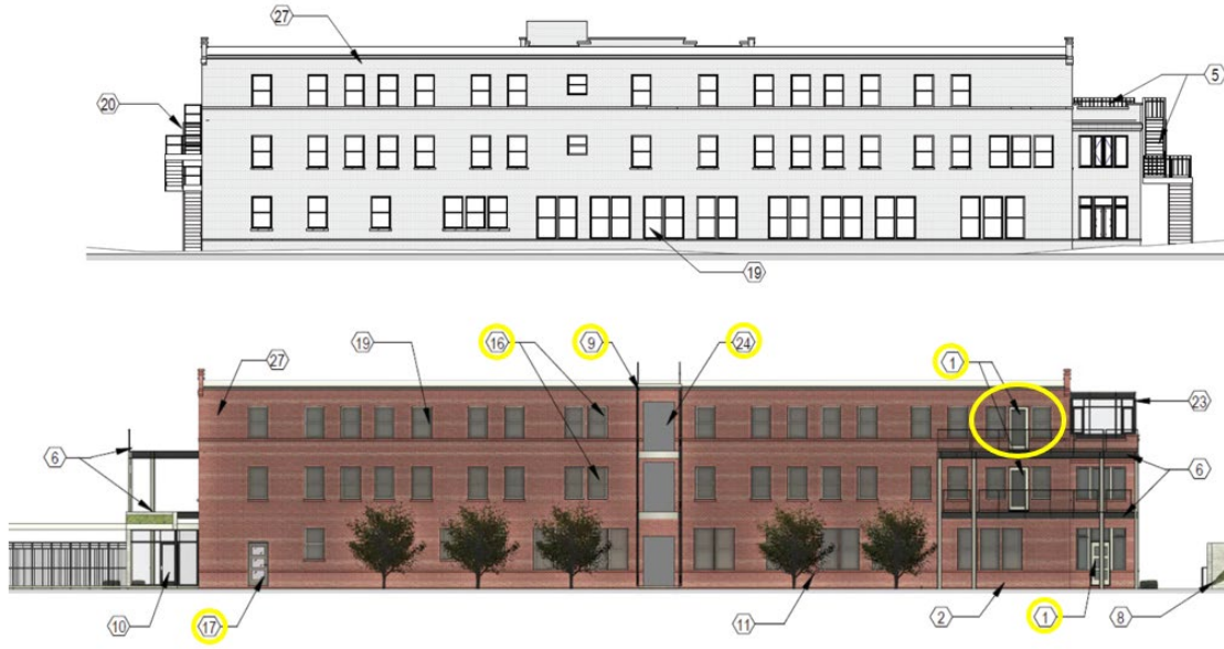
Figure 13. Existing (top) and proposed west elevation of 2543 4th St. Numbers noted in narrative highlighted. New window openings indicated by staff.
