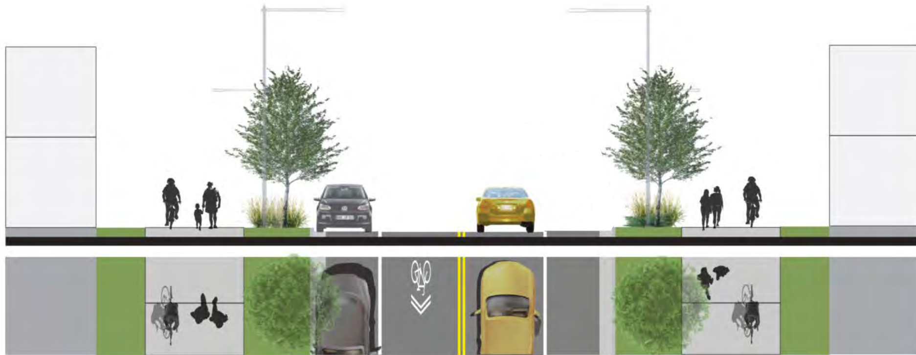
Commercial Street with Multi-use Path
