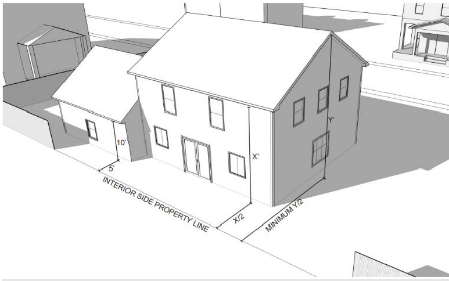
Figure 7-3: Setback Relative to Building Height
